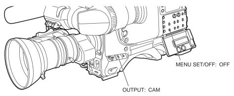
2 Press the AUTO W/B BAL switch to the ABB side and then release the switch. The switch returns to the center and the black balance is automatically adjusted.
